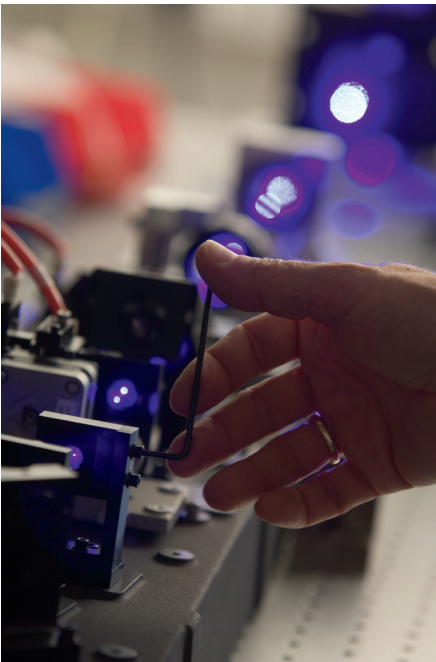
Fine-tuning of the violet laser beam profile gives the Luxel V-8 its outstanding hard dot characteristic for ultimate quality imaging (right). Precision engineering and alignment of the laser optics is the other half of the story (below).
